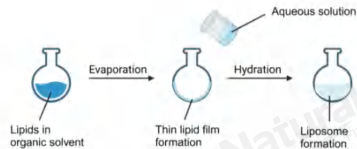
Figure 4. Demonstration of the use of the thin film hydration method to generate liposomes.
